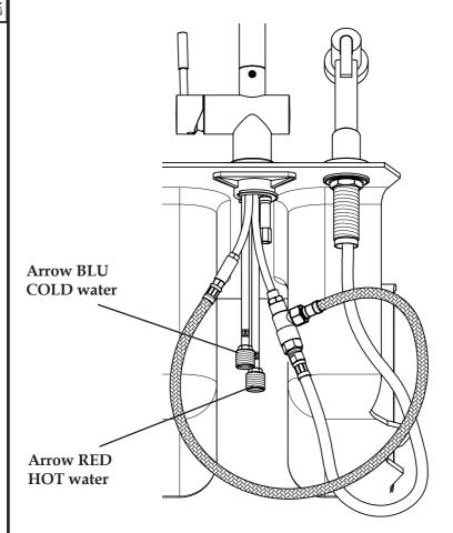
Connect the hot and cold supply lines. Do not allow the supply tubes to twist or bend sharply. Leave the valves closed.
